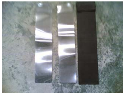
Figure: (3) Lead Screens.
